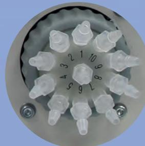
Pump distributor for 10 connections, controlled via the respective staining programm
