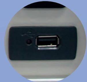
USB 3.0 for fast data transfer, e.g. for readout of completed staining protocols
